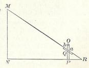
PQ was found by measurement to be 4 feet, RP 6 feet, PN 120 feet. Required MN.
