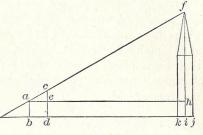
The similar triangles aec and ahf give us the proportion ae: ah:: ec: hf. What is the distance ec? ah = bi = bd + dk + ki.  $ki = \frac{1}{2}kj$ . When fhis found, what must be added to get the height of the tower?
